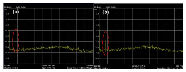
Figure. S1 The RF spectra of the TML mode and the corresponding unlocked states. (a) is the measured spectrum of the TML mode. And (b) is the unlocked states with a mode beat be measured.
